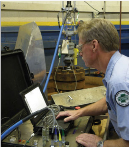
□ To diagnose pressure relief valves, technicians should have electronic valve testers that can test a valve in situ.
