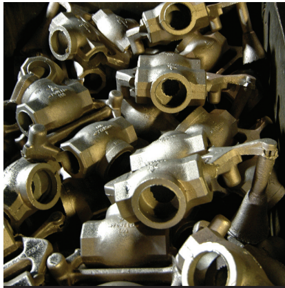
□ These bronze castings have been pre-cleaned in a shot-blasting machine. The next step will be to remove the sprues and smoothly grind away any burrs or surface aberrations.
