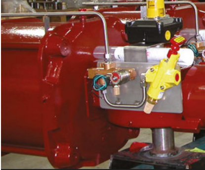
Fluid power direction control valve (gold color) with solenoid
