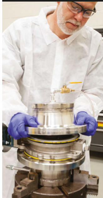
☐ Testing after clean assembly in Dezurik clean room
