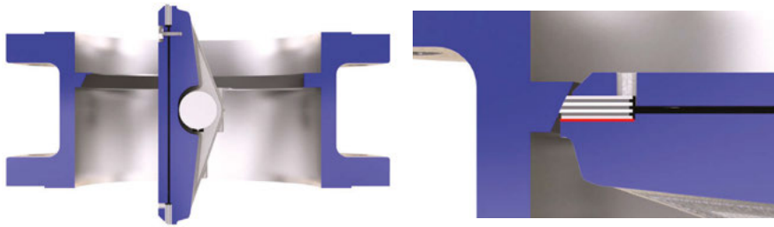
□ Figure 3. One of the benefits of using a wide gasket TOV is that it assures an even compression over the entire sealing surface of the laminated seal, resulting in a long seal life and tight shutoff.
