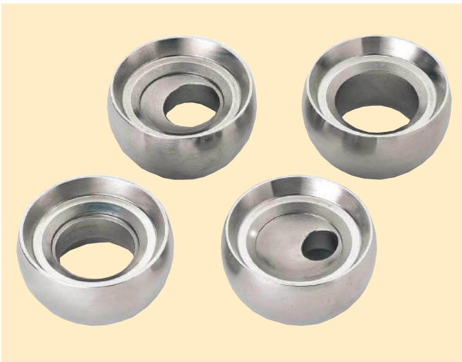
Figure 2. Four interchangeable seat trim sizes for a rotary control valve allowed a mine to increase capacity and maintain accurate control without replacing the valve body.
