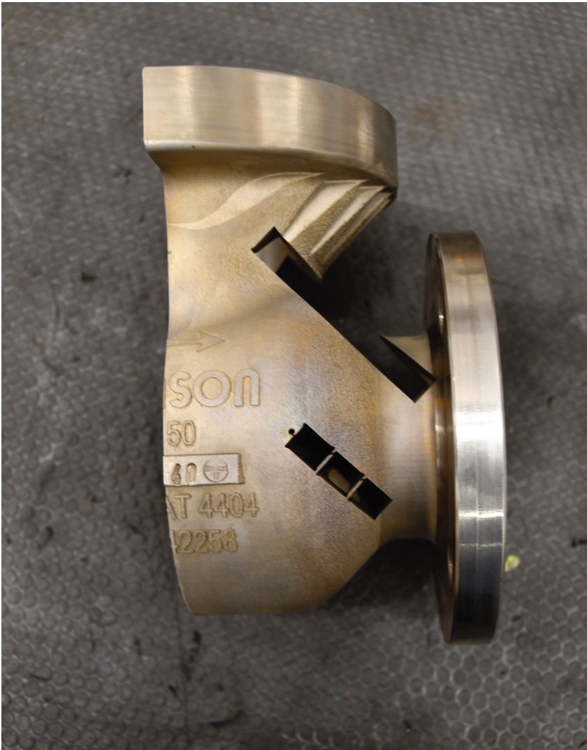
Examples of the additively manufactured samples. Source: SAMSON
