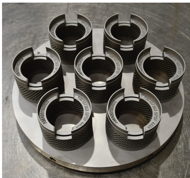
Top: Three-layer print of medium-sized plug heads (150 pieces).
