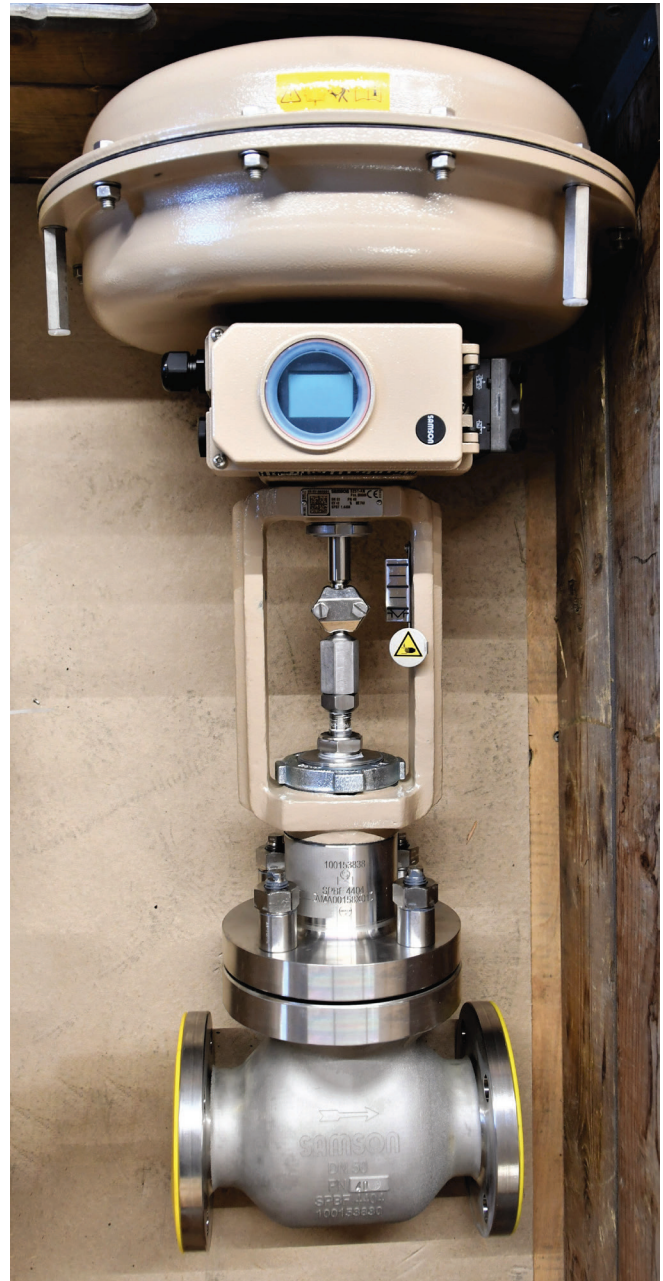
Additively manufactured pilot lot of DN 50 PN 40 valve, body and bonnet. Source: SAMSON
