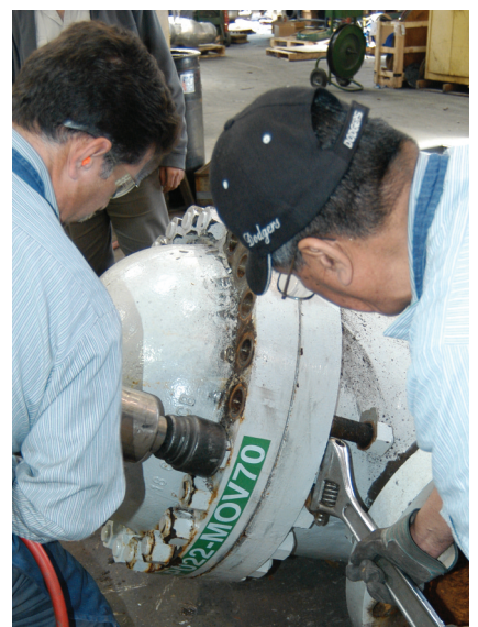
Workers disassemble a refinery valve prior to initial pre-repair inspection.
