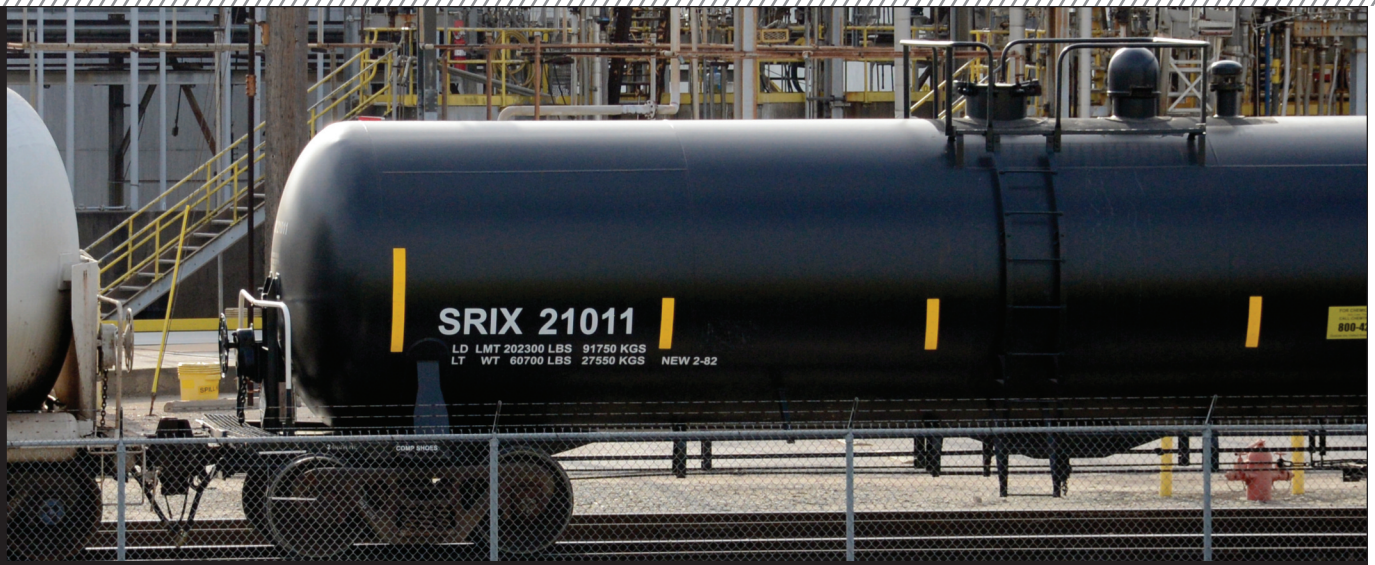
□ Tank cars generally have at least two sets of valves: inlet/outlet and a pressure relief valve.
