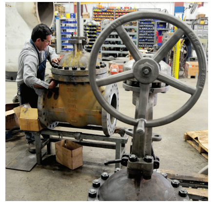
A chrome/moly block valve is disassembled in a VRC member company repair facility. Larger, higher pressure gate valves and alloy valves are still economical to repair, rather than replace.
