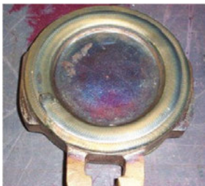
Figure 8. Wedge valve hardfaced with cobalt-based alloy
