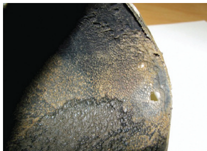
□ Figure 2. ABOVE: FAC damage in 2004 to Mihama Unit 4, which caused five fatalities and several injuries. BELOW: FAC damage to tube interior. Looking inside of a header tube shows FAC damage that occurred at tube bends. Courtesy: Tetra Engineering Group
