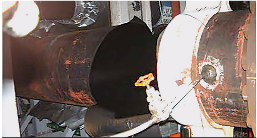
□ Figure 2. ABOVE: FAC damage in 2004 to Mihama Unit 4, which caused five fatalities and several injuries. BELOW: FAC damage to tube interior. Looking inside of a header tube shows FAC damage that occurred at tube bends. Courtesy: Tetra Engineering Group
