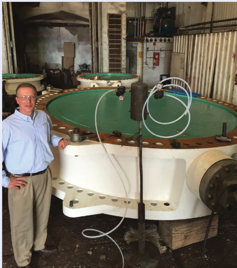
Figure 5. R. Scott Scheffler of MOOG Flo-Tork with new 102-inch butterfly valve.
