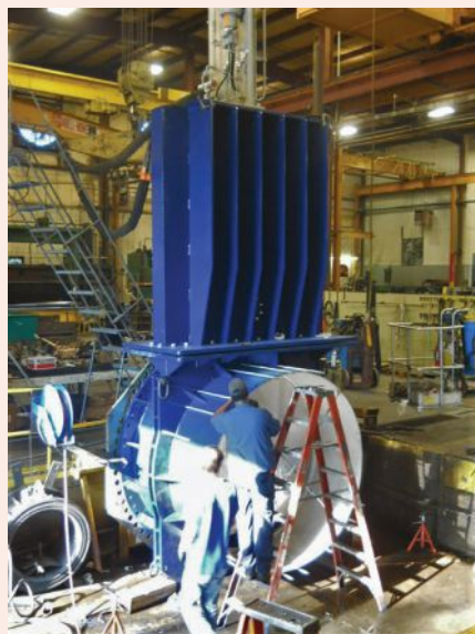
Figure 4. 84-inch knife gate valve.
