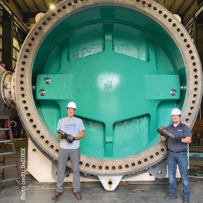
Figure 1. 168-inch AWWA butterfly valve.
