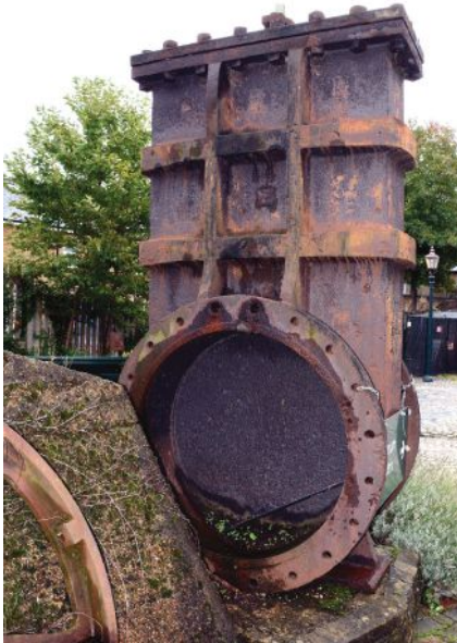
An example of the original wedge-style gate valve designed by James Nasmyth in 1843. This one dates from 1848-1850.
