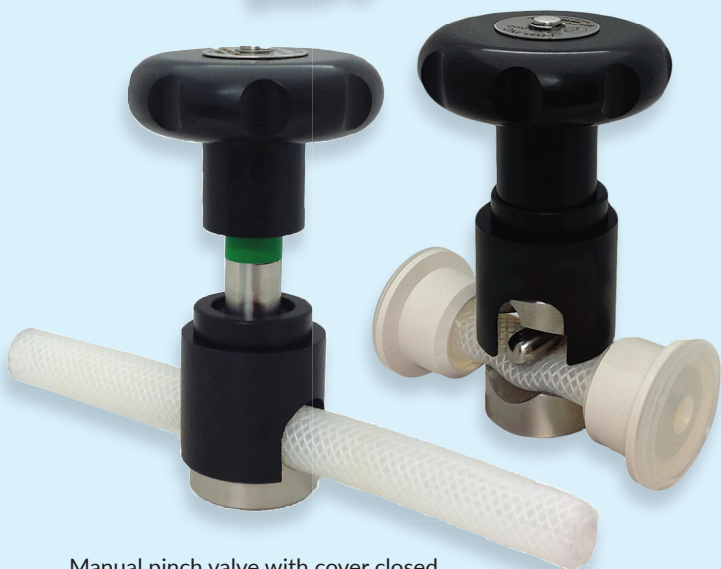
Manual pinch valve with cover closed (left) and open (right) to show hose compression.
