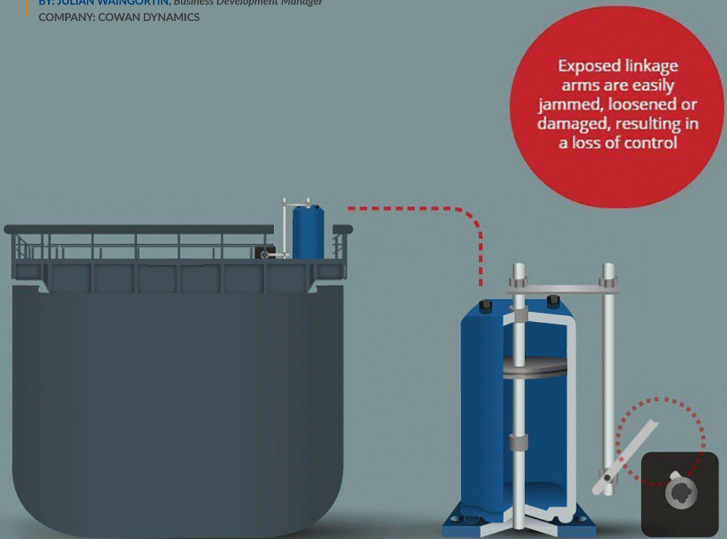
Figure 1: Linkage arm positioner in traditional actuators for dart valves in froth flotation cells.
