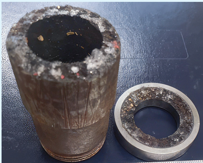
Figure 1A : Fractured cast iron yoke stem bushing made of D-2C material. All Photos: Velan Inc. (unless otherwise noted)
