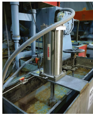
Figure 3: 150 psi pneumatic actuator with integrated position transducer. The position transducer is fully enclosed and protected from the corrosive surroundings in a flotation unit in a potash mine in Canada.
