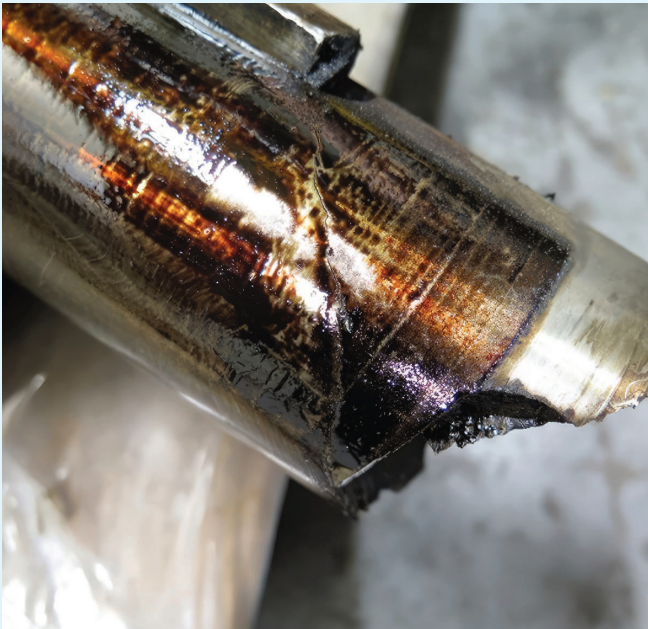
Figure 4: Brittle fracture of a17-4 PH stem in H1100 condition, likely caused by inconsistent heat treatment and exposure to a sour environment.
