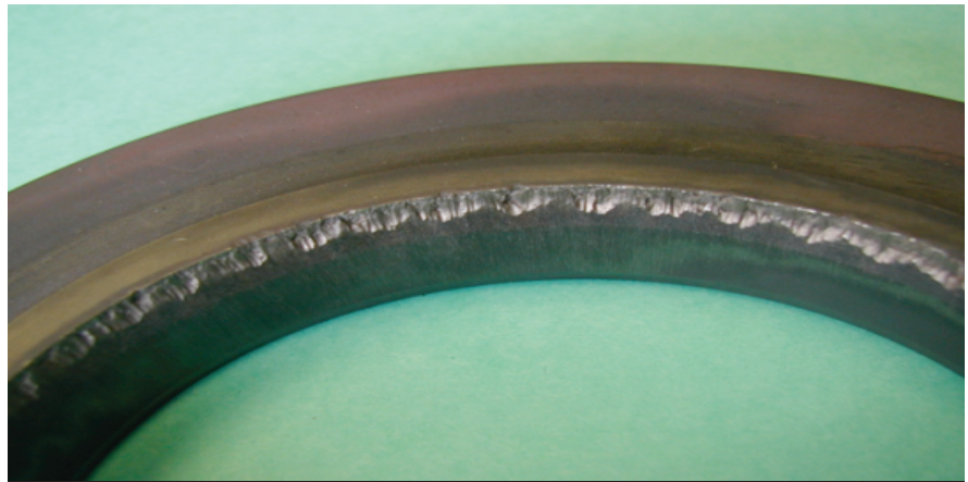
□ Figure 3. Valve seat ring damage due to operation of the valve below minimum throttling point, as well as damage due to the presence of particulate.
