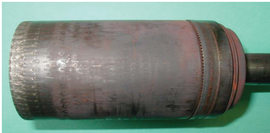
□ Figure 2. Valve plug damage resulting from operating below minimum throttling point, as well as damage due to the presence of particulate.
