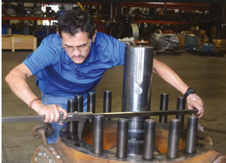
□ A metal-seated ball valve gasket pocket is measured to ensure that the OEM replacement gasket will fit properly.
