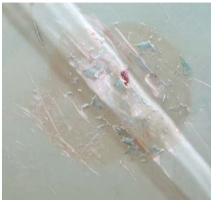
□ Figure 2. The abrading with sandpaper only covers a small portion of the entire area patched.
