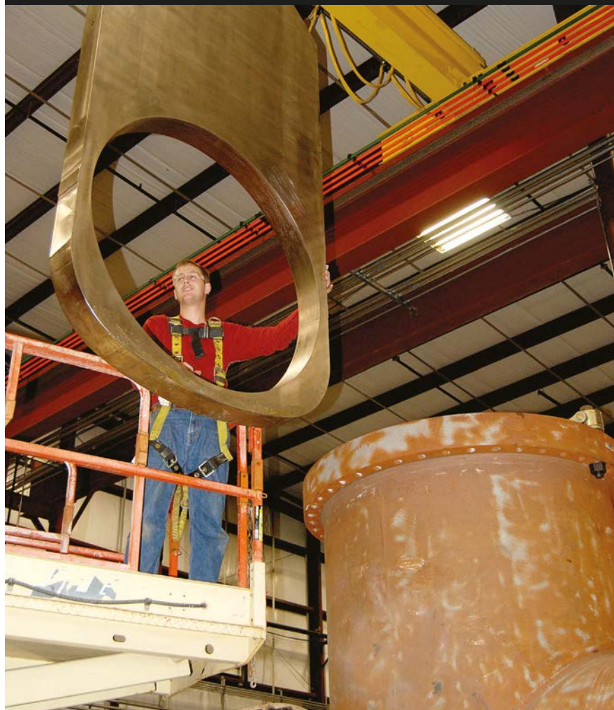
□ A 48-inch NPT, Class 600, reground gate valve disc is inspected prior to assembly. Grinding of discs are expenditures that can add to the price and delivery of a valve repair quote.
