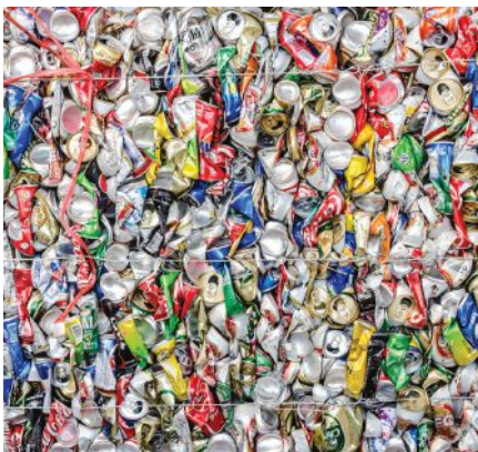
Recycled aluminum cans have a limited use. They cannot even be used to make new cans because of the impurities at the molecular level that affect the metal's strength, ductility, tensile strength and toughness values.
