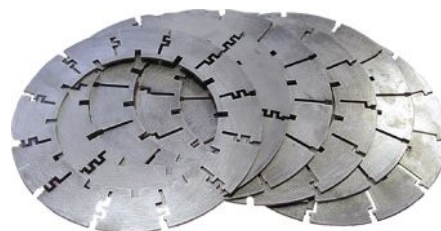
Figure 6. Laser-cut stack disks
