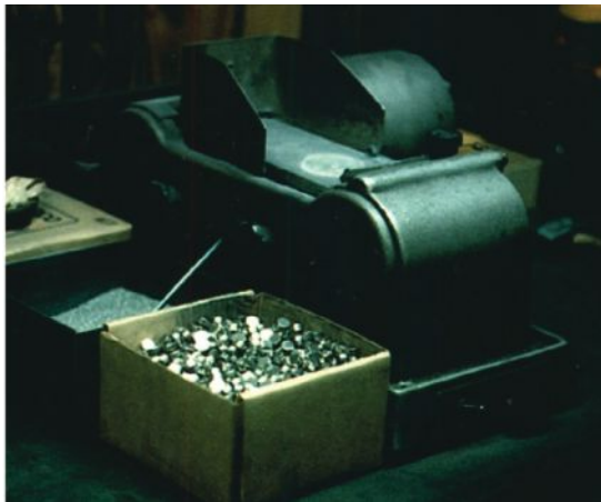
Two of these tablets of pure bismuth, each smaller than a penny, when added to 13 tons of molten white iron, would affect the iron's ability to be transformed to malleable cast iron when put in a 36-hour annealing furnace.
