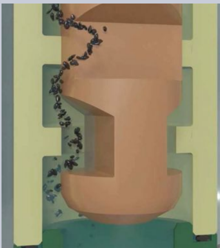
Figure 9. Non-compressible dirty service cavitation elimination
