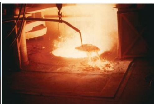
The author inspecting one of three 13-ton Brown Boveri Induction furnaces. Before a melt pour that occurred every 20 minutes, molten slag was skimmed off the surface of the furnace.
