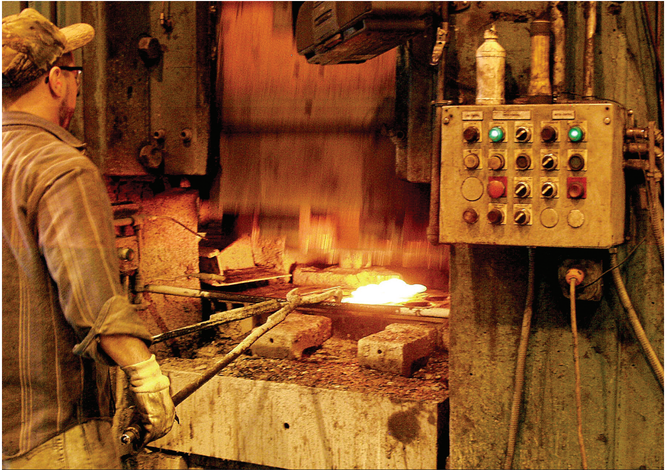
□ A small valve body is forged.
