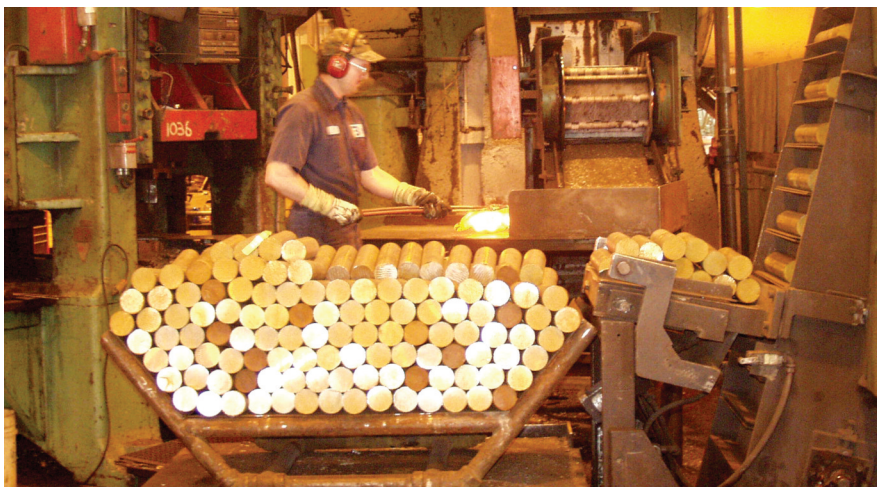
□ These billets have been pre-heated in preparation for forging.
