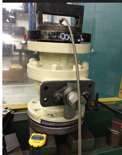
□ A ball valve being tested. Note the leak offline from the top of the valve, which is used to measure the leak rate during the internal test. The stopwatch is used to measure the test time.
