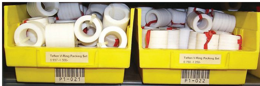
PTFE is used to manufacture packings for demanding corrosive services as well as ultrapure applications such as food preparation.
