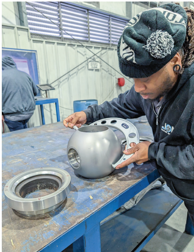
Inspection of chrome carbide-coated and lapped ball and seats.
