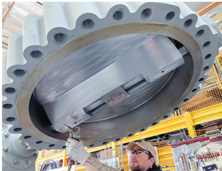
An employee of Curtiss-Wright works on a butterfly valve that will be shipped to a nuclear customer for installation in their plant. Source: Curtiss-Wright
