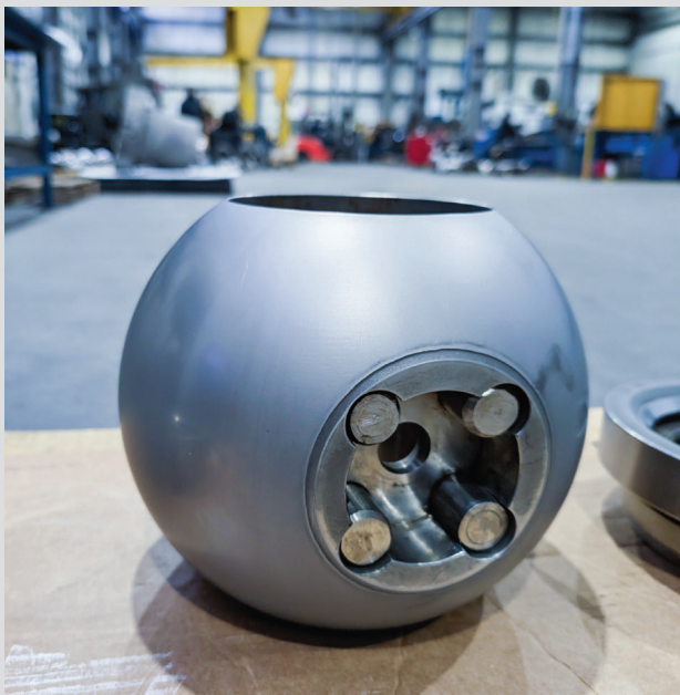
Lapped chrome carbide-coated ball before reassembly.
