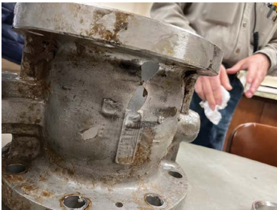
Large holes formed in the body of this valve after a few weeks in service.
